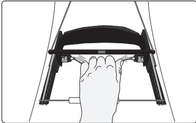
Pull the line behind the foot rest to release lock pins from the rail.
