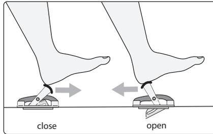
Open the bailer to drain any water out of the cockpit. Use your hand or one of your heels to push the lever back toward your body to "open" position. NOTE: Water will drain out only while the V7 is moving forward. If you are not moving or if you are moving in reverse, the water will go inside the cockpit.
